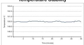
The drying chamber's temperature stability of  $\pm 0.5^{\circ}$ C ensures experiment stability.
