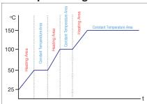
In program control mode, the controller allows the operator to set up step heating control.
