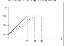
In program control mode, the controller allows the operator to set up linear ramp heating profiles.
