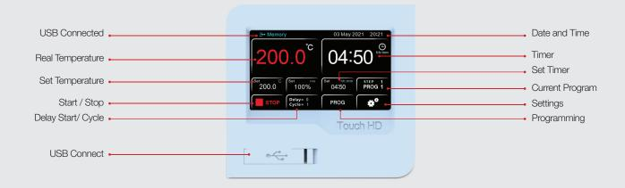
The BEING intelligent controller has a 4.3-inch color, easy-to-read, real-time touchscreen display to select the various functions with all the parameters — temperature, fan speed, time, program number, and step — on a single screen, providing quick and easy setting of temperature, time, and other parameters — and convenient operation.
