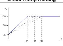
In program control mode, the controller allows the operator to set up linear ramp heating profiles.
