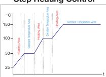
In program control mode, the controller allows the operator to set up step heating control.
