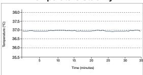
The incubation chamber's temperature stability of  $\pm 0.2^{\circ}$ C ensures experiment stability.
