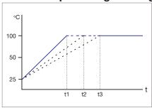
In program control mode, the controller allows the operator to set up linear ramp heating and cooling profiles.
