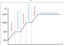
In program control mode, the controller allows the operator to set up step cooling and heating control.
